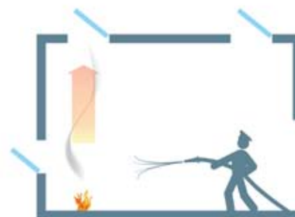
3. The smoke-free layer allows safe access for the fire to be fought and extinguished.
