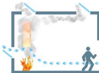
2. This allows cool air into the building forcing the hot air and smoke out via the roof, providing a smoke-free layer for safe escape.
