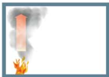
1. In the event of a fire, actuators open high-level smoke clearance units and low level fresh air inlet vents.
