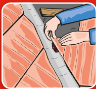
Adhering tiles or tile pieces to valleys
