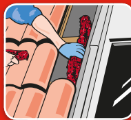
Adhering tiles to roof windows
