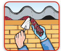
Sealing of corrugated roofs
