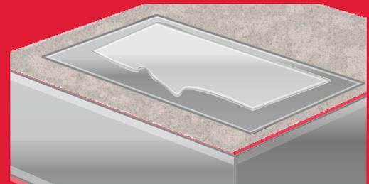
**Please ensure** that when applying Joint Tape that it is completely flat and free of gaps or fish mouths.
